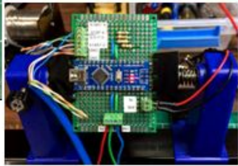
Model Railroad Speedometer Arduino Circuit—Part 1
